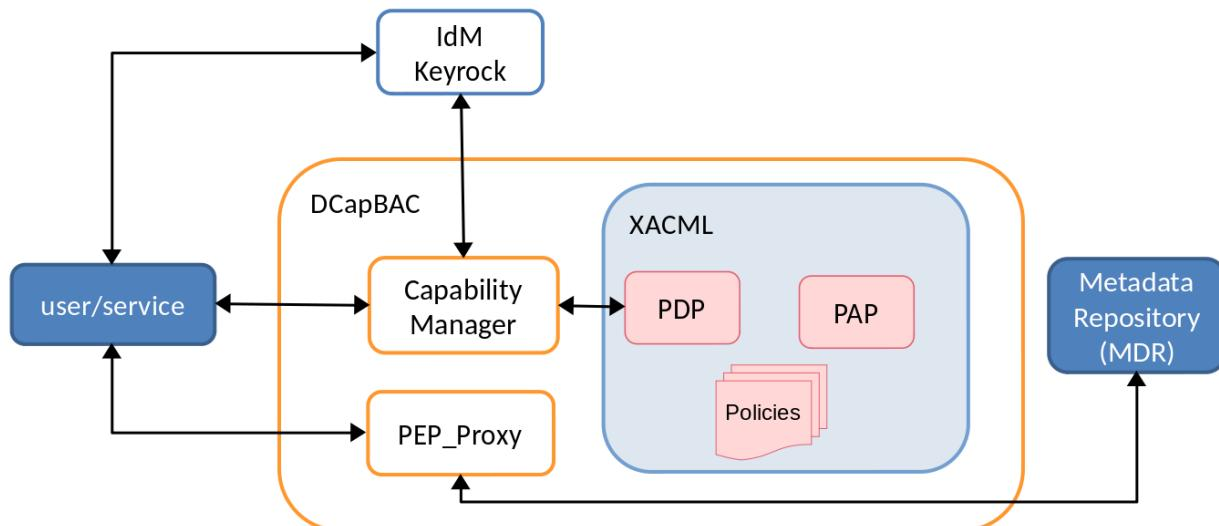
Remembering DCapBAC technology, where access control process is decoupled in two phases:
