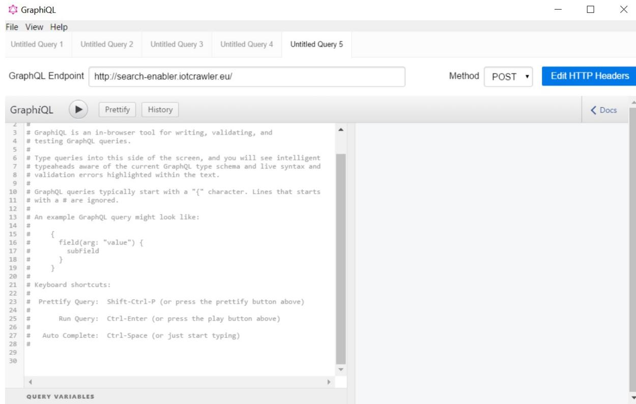
User assistance in GraphiQL is based on a GraphQL schema of a target endpoint. The schema describes the structure of a query language of target endpoint (data types, interfaces, queries, mutations).
